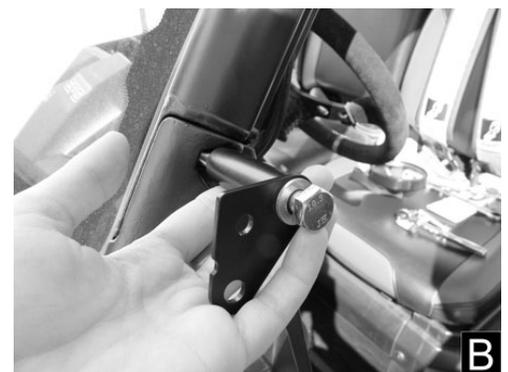
**Step 4:** Tighten upper bolt until snug enough to hold bracket out of the way of lower bolt. Remove lower bolt from A-pillar and discard. (Figure C)
