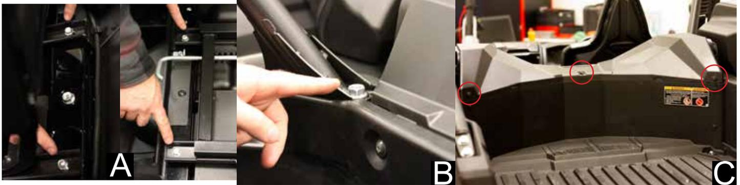
**Step 5:** Locate the 4 square plastic shapes located on the rear of the cockpit. **Figure-D**
