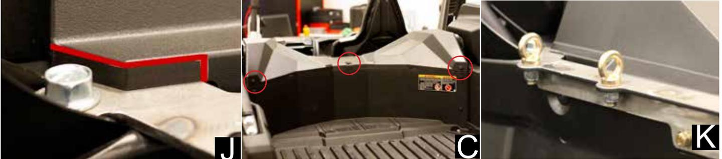
**Step 11:** Now that you have your harness brackets installed you can remove your factory seat belts and install the harnesses. First you will remove the factory seat belts and **keep the outer lap mount bolts** for later. We provide two bolts and spacers for the inner lap-mounts.
